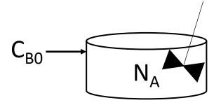
Caution:  $C_{B0}$  is the concentration of B entering the reactor, NOT the initial concentration of B.
