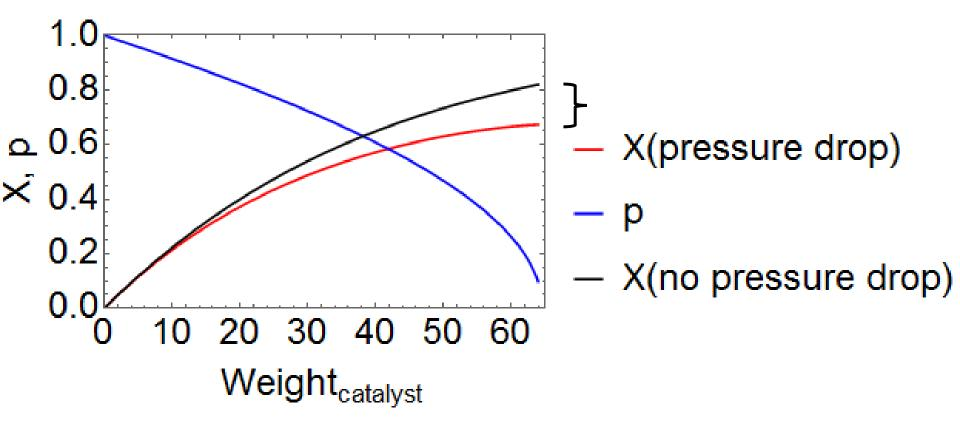
About 15% drop in conversion indicated. Could be millions of dollars in unpredicted losses (less ethylene oxide made) if pressure drop is not accounted for.
